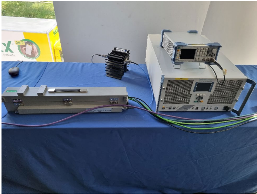
Figure 33 Close up view of the EMI clamp and amplifier
