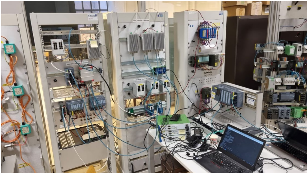
Figure 37 The PN TSN test bed: (middle, top to bottom) 3 Relyum, 3 Phoenix Contact and 3 NXP TSN bridges; (left and on the table) measurement tools and PN devices
